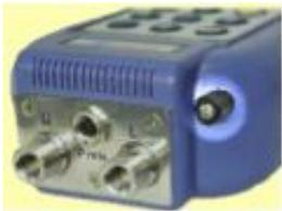
Pressure media: AISI 316 SS compatible fluids (water, gas, and oil)
