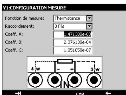
With 50 Kohms range and Steinhart – Hart equation integrated, thermistors can be entered into CALYS 150 and tested. Steinhart-hart equation is as follows:  $1 = A + B(\ln(R)) + C(\ln(R))^3 T$  Where: A, B and C are usually calculated according to temperature at 0°C, 25°C and 70°C
