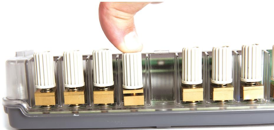
Connect your probes by simply pushing on the terminal top and insert wires of up to 3 mm or 10 AWG diameter and compensated thermocouple connectors. Wires are held tight between two brass plates ensuring thermal stability and a very good cold junction compensation for thermocouples. This system also enables 4 mm banana plugs and security connectors to be connected on the terminal top.
