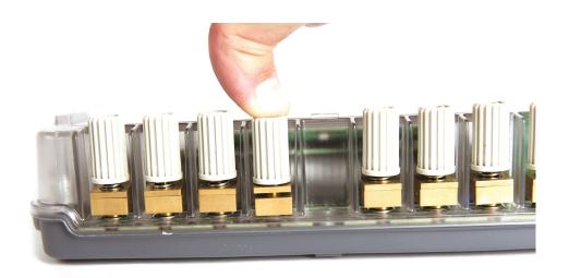
Connect your probes by simply pushing on the terminal top and insert wires of up to 3 mm or 10 AWG diameter and compensated thermocouple connectors. Wires are held tight between two brass plates ensuring thermal stability and a very good cold junction compensation for thermocouples. This system also enables 4 mm banana plugs and security connectors to be connected on the terminal top.
