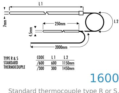
Standard thermocouple type R or S, for Primary laboratory, 0°C to 1600°C
