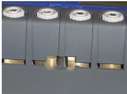
Connect your probes by simply pushing on the terminal top and insert wires of up to 3 mm or 10 AWG diameter and compensated thermocouple connectors. Wires are held tight between two brass plates ensuring thermal stability and a very good cold junction compensation for thermocouples.
