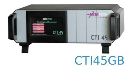
CTI45 Ohmmeter, Insulation Megohmmeter, microhmmeter
