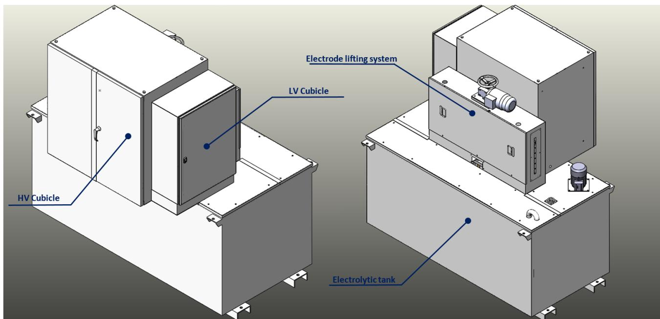
Each starter is offered with an agitator system (propeller or pump) to ensure the thermal and chemical homogeneity of the electrolyte. Thermostats and a level sensor are installed to ensure the safety of the starter.
