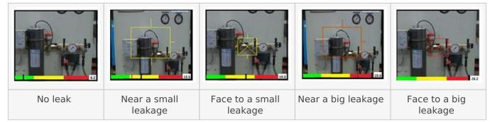
The LEAKSHOOTER LKS1000 V.2 is used like a camera. When it comes near a leak, a dynamic yellow target appears on the large colour screen. The target turns red and shrinks as it approaches the source of the leak. A bar graph at the bottom of the screen accompanies and facilitates the search.
