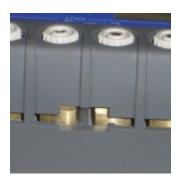
Connect your probes by simply pushing on the terminal top and insert wires of up to 3 mm or 10 AWG diameter and compensated thermocouple connectors.
